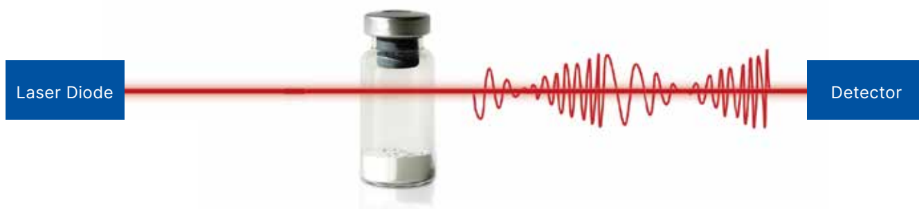
Diode laser light being transmitted through a container for headspace characterization.
